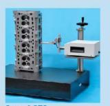
Stand ST2 Code: 1401 Stand ST2 is made up of a 630x400 mm granite base and a positioning column. It reaches a maximum height from the plane of 250 mm. It is suitable for the translator TS7 and TL90.
