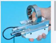
The compact and handy TS7 can perform neasurements even in the most difficult conditions olding it with just one hand. The probe can be rotated 90 degrees and the height
