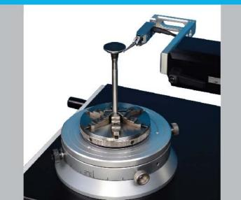
The software allows to analyse the following geometrical tolerances: roundness, straightness, cilindricity, conicity, cone form, concentricity, parallelism, coaxiality, run-out, total run out, thickness variation.
